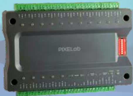
IEC3016 - Elevator Floor Control Unit
